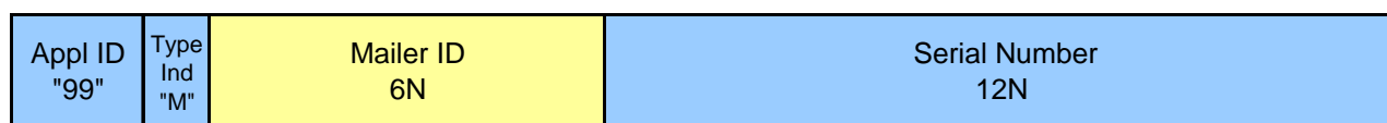
Figure 12. Field Layout of the Intelligent Mail Container Barcode with 6-Digit Mailer ID
